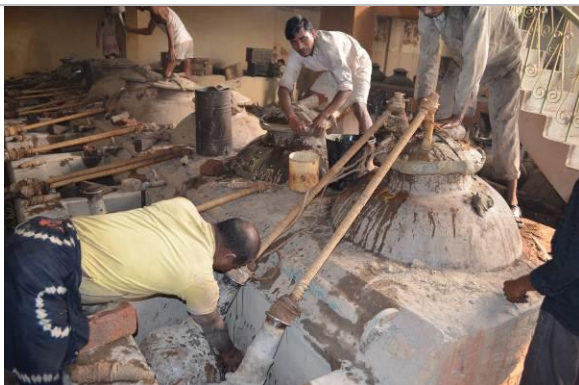
Chongas fixed and made airtight with multani mitti
