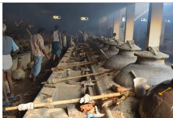
Chongas to connect the Deg and the Bharka
