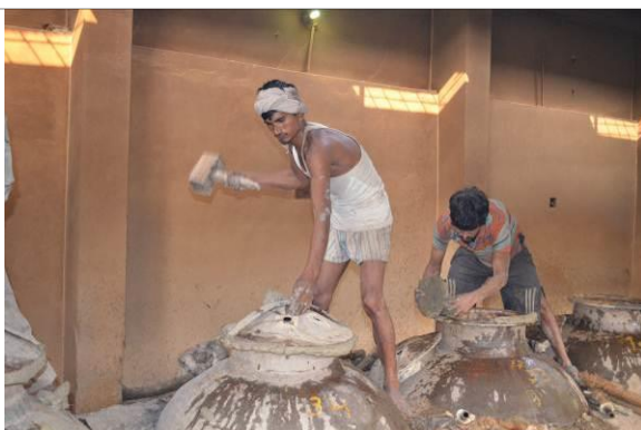
Deg is secured and made air tight
