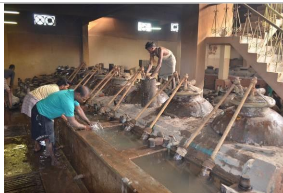
Chongas fixed and made airtight with multani mitti
