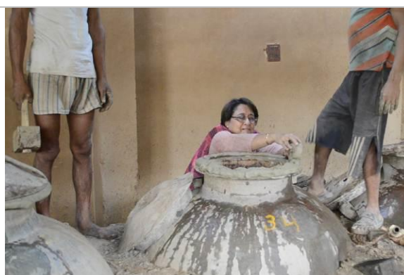
Deg is sealed with 'Chikini Mitti'
